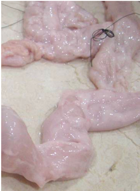
Fig. 1 – Pressure resistance test. Three-hundred and fifty segments of porcine large bowel measuring 60 cm were washed and prepared in order to remove external fat and internal feces.
